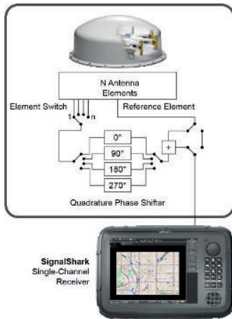
Fig. 5. Direction finding principle
