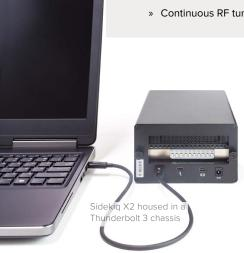
Sidekiq X2 can be integrated with a COTS FPGA carrier card that includes a GPSDO card integrated into a Thunderbolt<sup>™</sup> 3 chassis or, for ruggedized deployments, into COTS 3U or 6U VPX carrier cards. Conduction and convection cooled options are supported. Sidekiq X2's Platform Development Kit (PDK) provides access to both a software API for interfacing to the card, as well as the source code for the FPGA reference design targeting a Xilinx Kintex® UltraScale<sup>™</sup> XCKU060 device.
