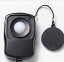
Silicon diode sensor and filter are designed for indoor use.
