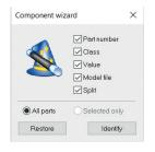
A component wizard is provided to simplify the component modeling, automatically identifying device classes, importing any available models and extracting valuable component information, such as value, tolerance, shape etc, directly from the BOM description.
