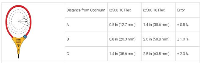
Measurement uncertainty assumes centralized primary conductor at optimum position, no external electrical or magnetic field, and within operating temperature range.
