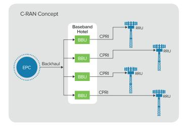
C-RAN simplified the backhaul network because several BBUs could be co-located together and served by a common, high-bandwidth connection. It also simplified synchronisation since all the BBUs could be served by the same time and frequency reference, guaranteeing accurate synchronisation.
