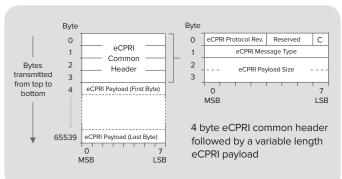
**C** (the LSB in byte 0) is the eCPRI messages concatenation indicator. A value of "1" indicates that another eCPRI message follows this one within the eCPRI PDU. A value of "0" indicates that the eCPRI message is the last one inside the ECPRI PDU.
