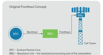
RRU - Remote Radio Unit - the RF transceiver part of the basestation
