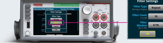
A moving filter will only delay the first reading by the number of user selected filter counts.
