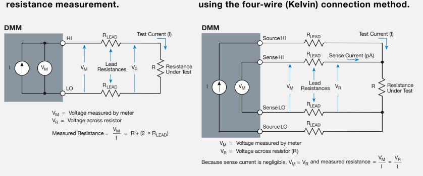
The effect of test lead resistance can be reduced using the four-wire (Kelvin) connection method.
