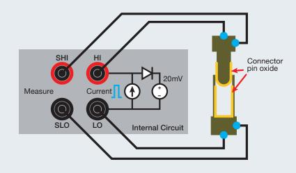
Low open-circuit voltage prevents puncturing oxide films, giving more realistic resistance measurements in connectors, relays, µP sockets, etc.
