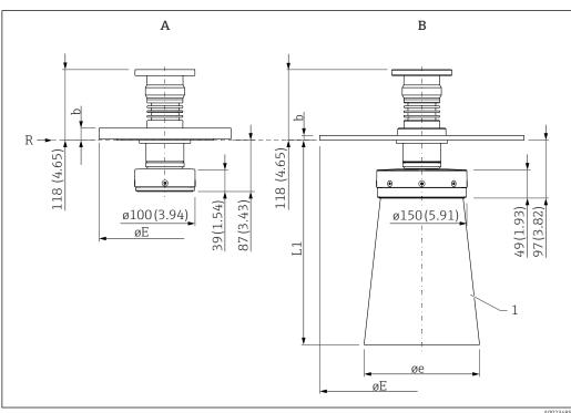
Dimensions of the planar antenna (NMR84); unit of measurement: mm (in)
