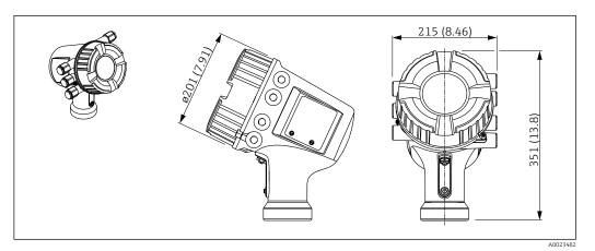
Dimensions of the electronics housing; unit of measurement: mm (in); adapters for cable entries are not taken into account in this drawing.
