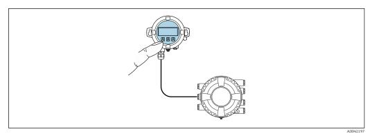
$\blacksquare$  18 Operation via remote display and operating module DKX001
