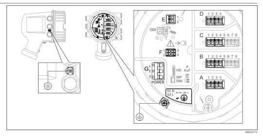
■ 9 Terminal compartment (typical example) and ground terminals
