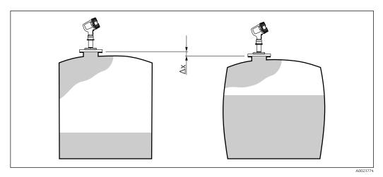
■ 21 Movement Δx of the Gauge Reference Height due to the bulging of the tank shell caused by hydrostatic pressure
