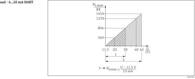
1 Supply voltage 11.5 to 30 V DC for intrinsically safe device versions (not for analog)
