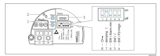
1 Operating keys for lower range value (zero) and upper range value (span)
