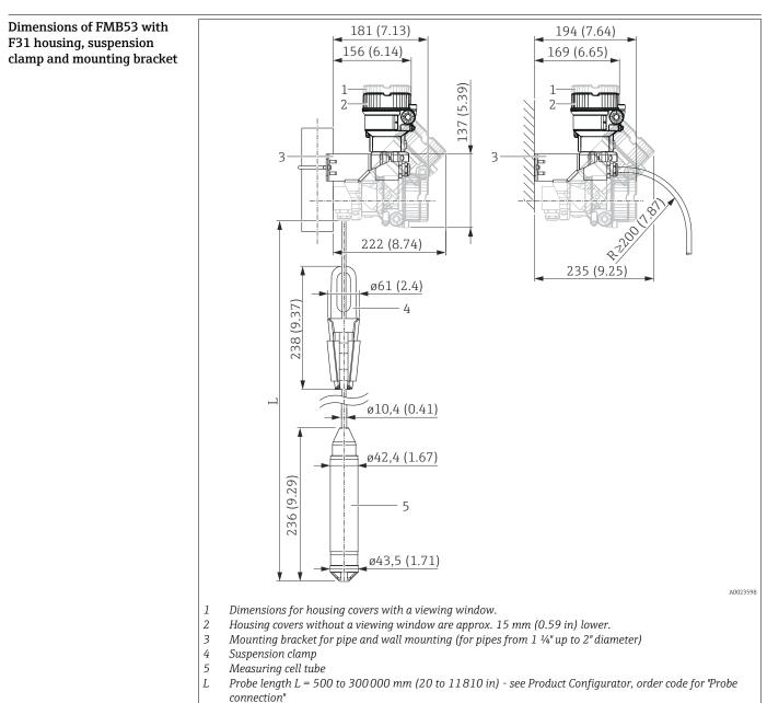
FMB53 with suspension clamp and mounting bracket (mounting bracket without marine approval) Engineering unit mm (in)
