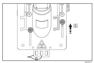
2. Slide the calibration plate into the radiation path to the upper limit stop.
