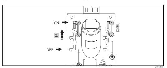
2. Using the bow-type handles, move the shutter (lead shielding) from the OFF position to the ON position.
