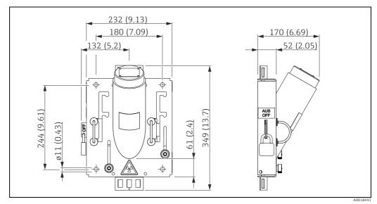
Dimensions: mm (in) Feature 240 "Emission Angle; Application", Option model 4 " 20 deg; density 30 deg diagonal radiation"  $30^\circ$  diagonal irradiation,  $20^\circ$  radiation emission angle
