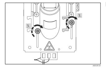
3. Tighten the clamps again. Perform the recalibration.
