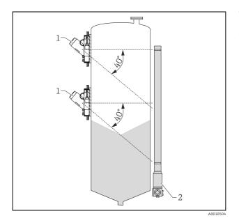
Two or more source containers are used for large measuring ranges. The use of several sources can be necessary not only from the aspect of large measuring ranges but also for accuracy reasons.
