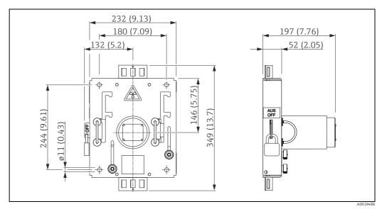
Dimensions: mm (in) Feature 240 "Emission Angle; Application", Option model 3 "20 deg; limit switch + density"  $20^\circ$  radiation emission angle
