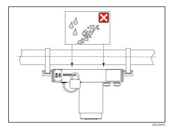
To guarantee the operation of the switch-ON/switch-OFF function, upside down installation or similar is only permitted if it can be ensured that no particles or high-viscosity liquids can enter the area of the shutter (see graphic).
