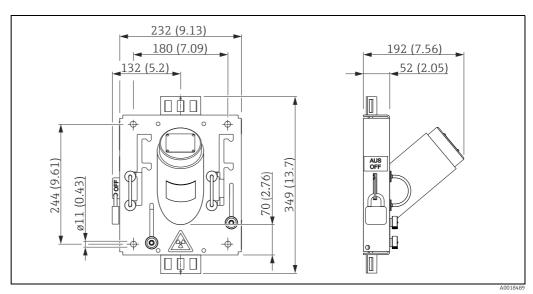
Dimensions: mm (in) Feature 240 "Emission Angle; Application", Option model 5 " 40 deg; level"  $40^\circ$  radiation emission angle
