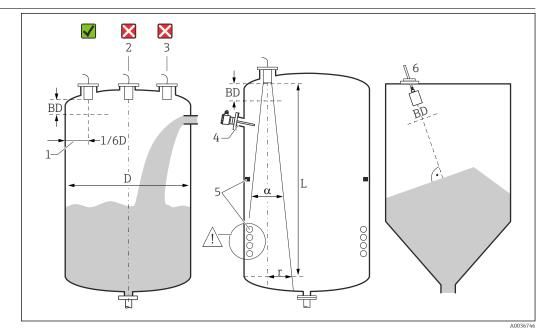
■ 5 Installation conditions for level measurement
