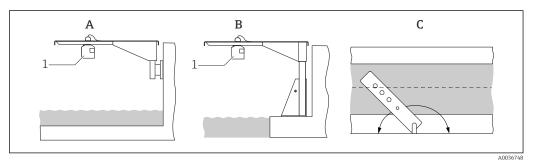
**₽** 7 Installation with cantilever arm over open channels or flumes
