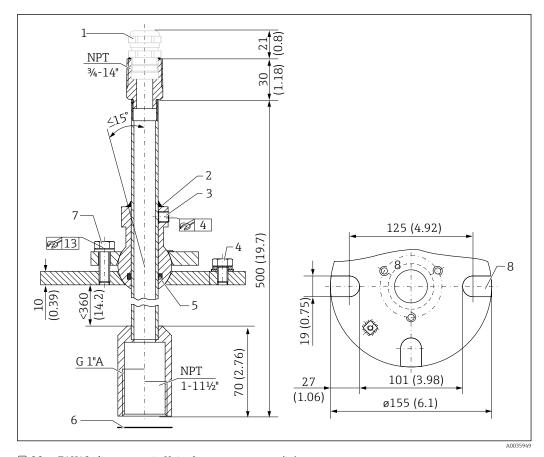
🗷 20 FAU40 alignment unit. Unit of measurement mm (in)
