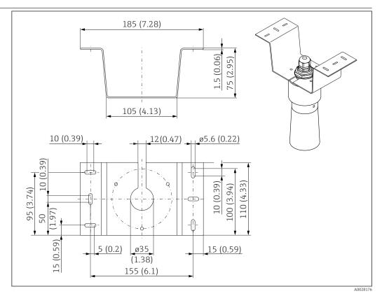
Mounting bracket for ceiling mounting. Unit of measurement mm (in)
