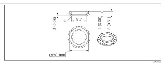
$\blacksquare 10$  Counter nut; dimensions. Unit of measurement mm (in)
