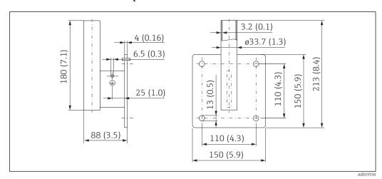
$\blacksquare$  18 Dimensions of the wall bracket. Unit of measurement mm (in)
