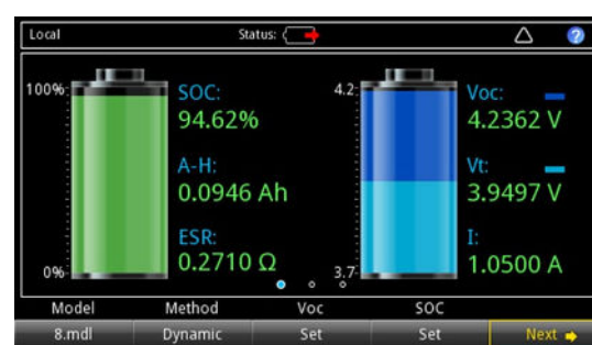
Figure 2. Battery simulator home screen.
